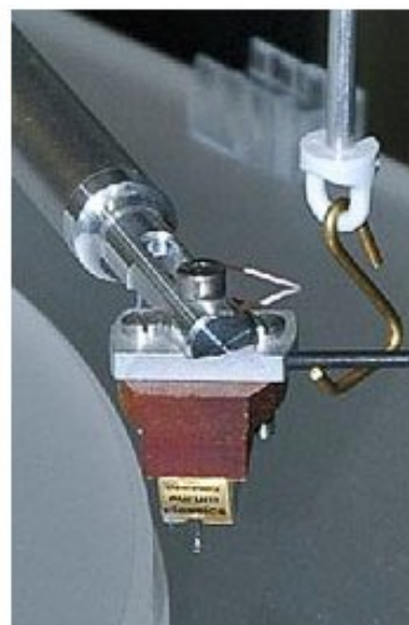
High-End turn tables Determine the bearing force of pick-ups
